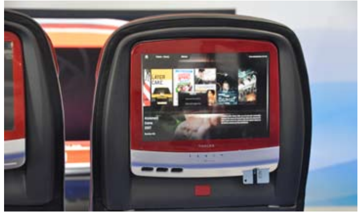
above: the new 12.1" monitor integrated into B/E seat
