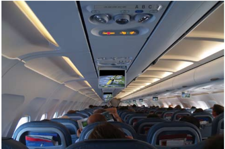
above: dPaves installation showing drop down monitor and Airshow
